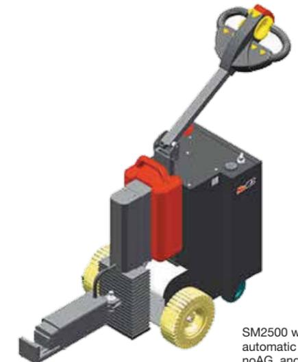
SM2500 with optional automatic gripping device part noAG, and automatic height adjustment device part noAH
